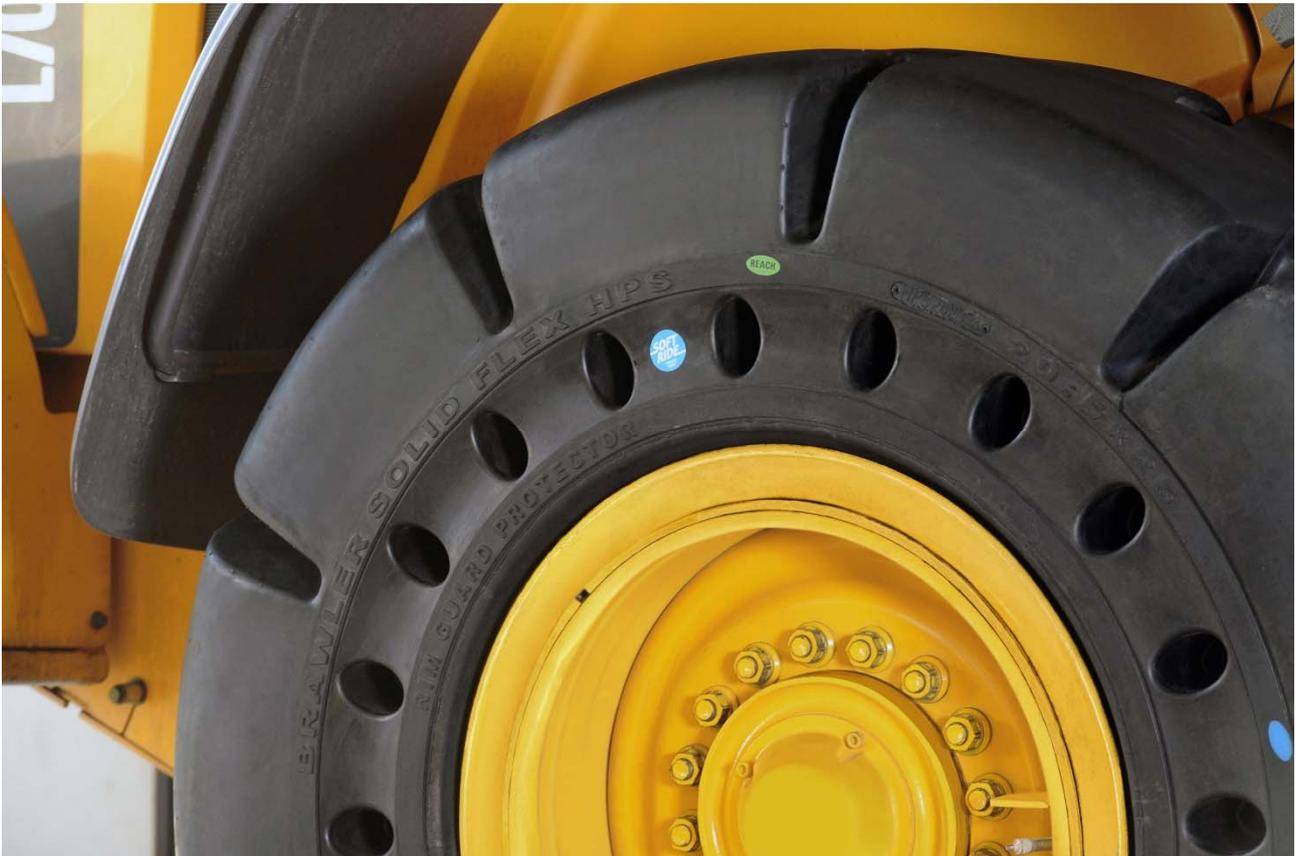
The Brawler HPS Soft Ride, a new solid tire designed and developed specifically for the waste management and recycling industries. (Photo Trelleborg Wheel Systems, TWSPR011)
