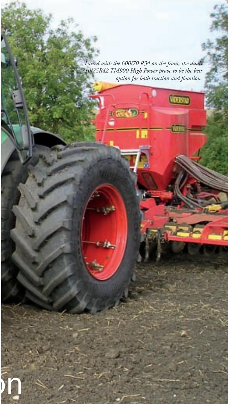
*Paired with the 600/70 R34 on the front, the duals 710/75R42 TM900 High Power prove to be the best option for both traction and flotation.*
