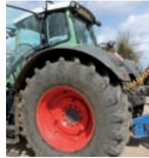
*Tall 710/75 R42 TM900s allow more wheel weight to be added to the farm's Fendt 936, putting more cleats in contact with the ground.*
