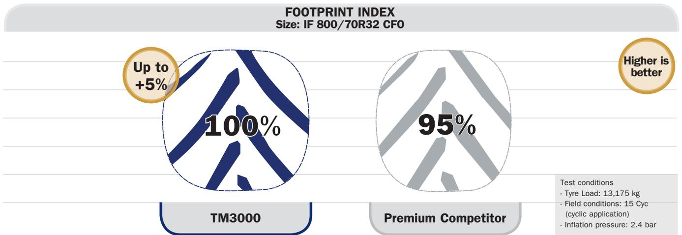
The larger contact area of the TM3000 significantly reduces soil compaction. The wide footprint area provides better flotation
