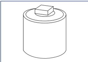
Valve guard, type **V3**. To be used when there is a greater possibility of impact. This style of valveguard fits all forestry and agricultural wheels. Its normal area of application is on forestry and construction equipment.
