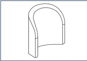
Valve guard, type **V1**. Normal area of application is on wheels intended for use in agriculture. V1 valve guard fits rims up to 26.5".
