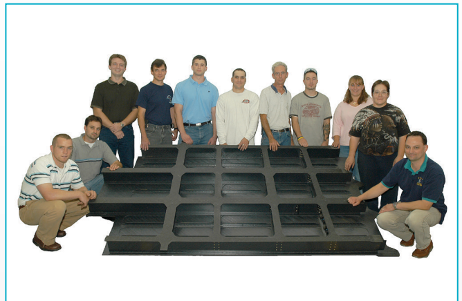
Figure 9: Fusion bonded helicopter tub structure
