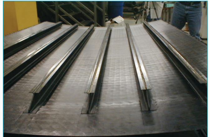
Figure 6 - Dassault fusion bonded skin/stringers
