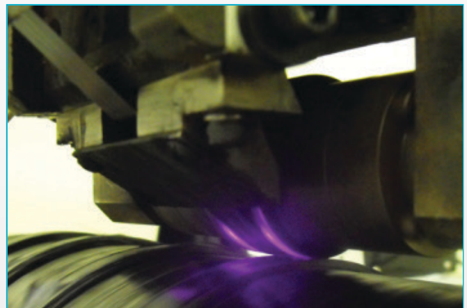
Figure 7 - Laser heating in TPC AFP
