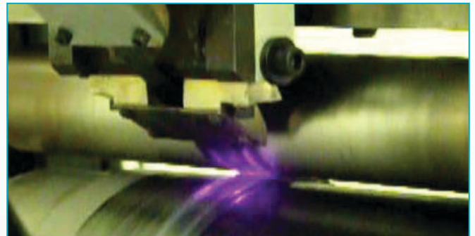
Photo 12 - Laser processing of CF/PEEK
