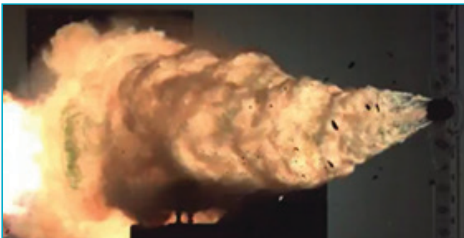
Photo 11 - Projectile being fired by electromagnetic powered railgun
