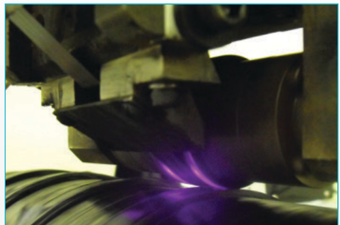
Figure 10 - Laser heating in TPC AFP
