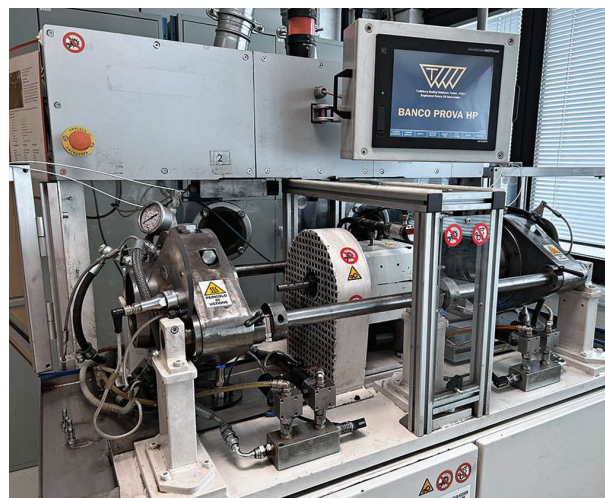
THE HPROS ADVANCED TEST RIG USED BY TRELLEBORG OFFERS MORE CAPABILITIES FOR TESTING SEAL OPERATING PARAMETERS SUCH AS TEMPERATURE, SPEED, TORQUE, PRESSURE, PRESSURE SPIKES, AND SIDE LOADS.
