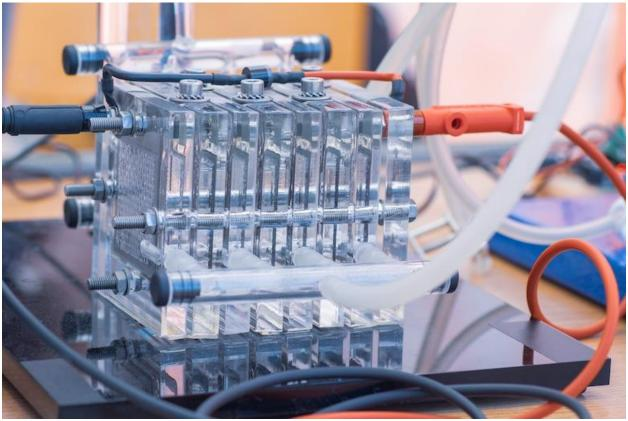
*Electrolysis which is a chemical process that separates hydrogen and oxygen molecules of water using electricity. Hydrogen produced by electrolysis can result in zero greenhouse gas emissions, depending on the source of the electricity used.*
