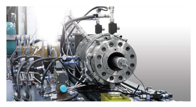
This test rig uses a three-dimensional accelerometer to measure vibrations from stick-slip operation between a rod seal and a piston seal and their respective mating surfaces.
