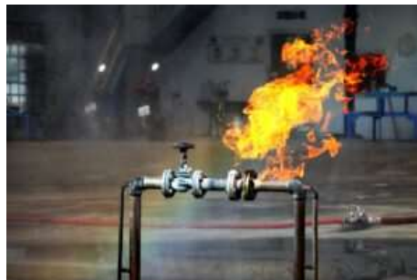
FIGURE 3. There are test standards available to test valves in fire situations
