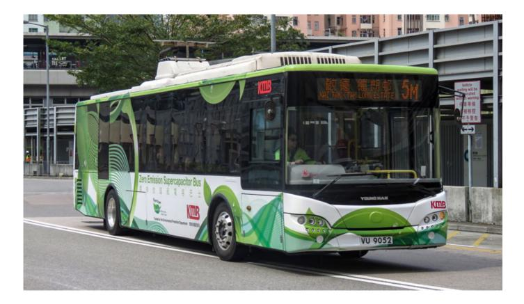
This bus in Shanghai uses ultracapacitors that allow fast charging. The buses is only able to travel three to five miles between charges. However, for urban areas, the buses can keep running with a fast recharging at designated bus stops.
