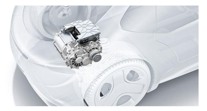
The e-Axle is a compact, cost-attractive electric drive solution for batteryelectric vehicles and hybrid applications. The electric motor, power electronics, and transmission are combined in a compact unit directly powering the vehicle's axle. Additionally, the powertrain becomes cheaper, more compact, and more efficient. (Credit: Bosch Mobility Solutions)
