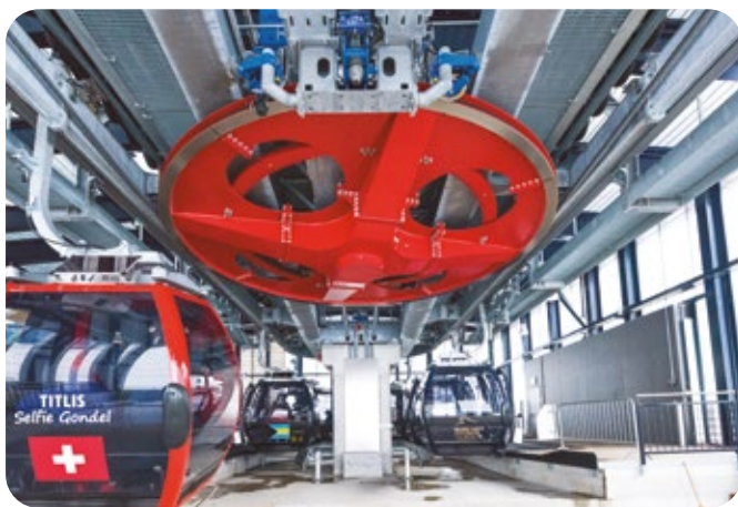
The monocable system is supported by a hydraulic cylinder that manages tension on the cable and smooths movement.
