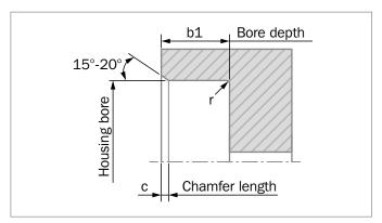
Figure 13: Housing design schematic
