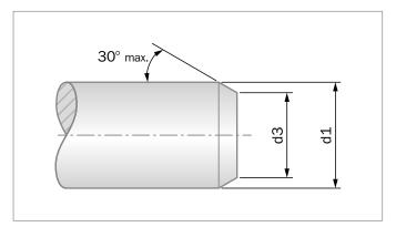
Figure 14: Shaft lead-in chamfer
