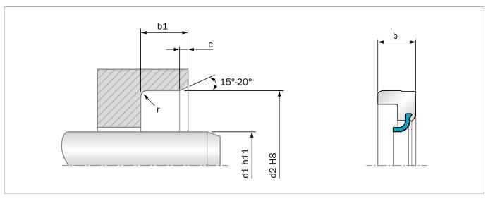
Figure 19: Installation drawing for pressures up to 0.5 MPa (73 psi)
