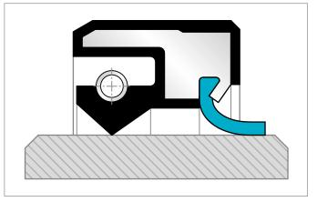
Figure 7: Elastomer/Turcon® Hybrid. This combination utilizes the best attributes of both a Radial Oil Seal and Turcon® Varilip® PDR.
