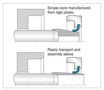
Figure 16: Assembly tooling types for installation on shafts
