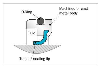
Figure 3: O-Ring Design. For low interference fits in the housing. Housing surface finish > 0.8  $\mu$ m Ra or particularly searching media control.
