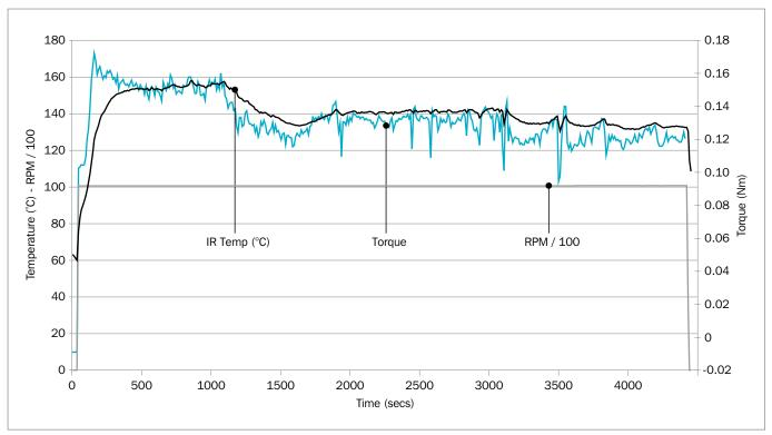
Figure 10: Running torque for Turcon® Varilip® PDR
