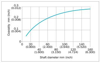
Figure 12: Coaxial tolerance capability
