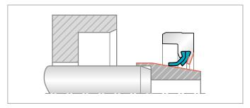
Figure 18: Ensure there is sufficient clearance between the support leg and the assembly cone
