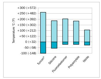
Figure 9: Maximum and minimum temperatures for different materials
