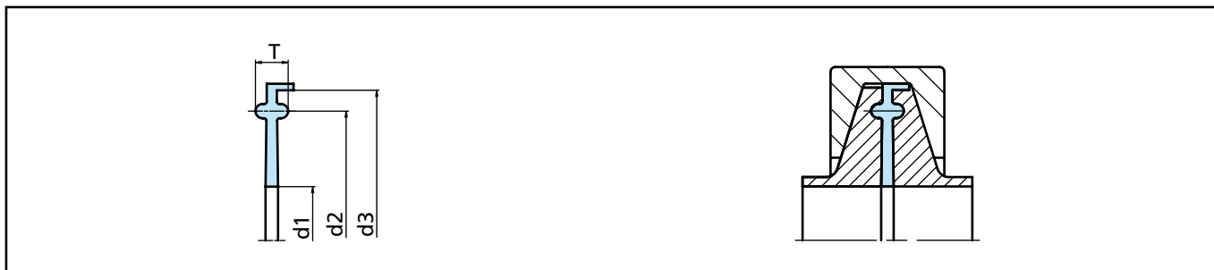
Figure 3 Seal dimensioning and installation
