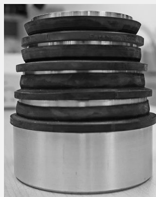
Forsheda® V-Ring in N6T50 strained at 10%, 20%, 30%, and 40% showed no cracks at any strain levels after 24 hours with ozone exposure.
