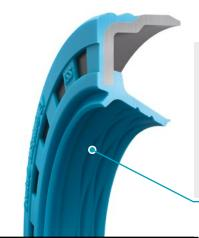
The PSW hydrodynamic texture on the sealing lip is designed to actively pump fluid back to the oil side during shaft rotation, regardless of the direction of rotation. This unique feature prevents leakage, enabling the Stefa® HiSpin® EV40 to effectively seal at shaft surface speeds of up to 40 m/s.
