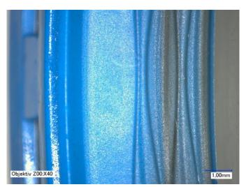
Inspection of seal after endurance test shows no signs of wear.
