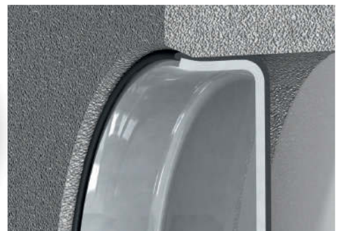
Cross section of a Rubore® Cap Seal
