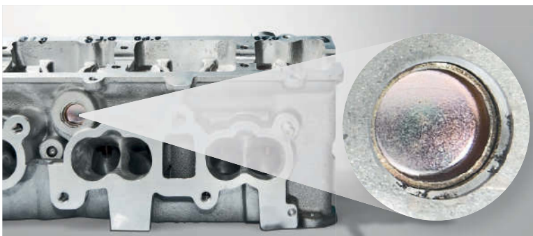
Camshaft housing with mounted sealing cap
