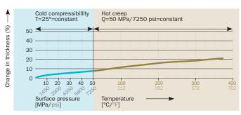
A precise description of the temperature test can be found in FlatSeal  $^{\text{TM}}$  Guide 10.
