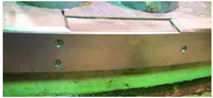
ment self-lubricating bearings, plant operator First Hydro Company designed a stainless steel liner to be attached to the track, as shown in the photograph on the right, that provided a hard, smooth surface with no corrosive activity.
