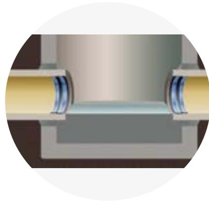
The compressive force providing the seal on either side of the joint is the result of increasing the effective diameter of the stainless steel expansion bands. The patented Slotted Band® is constructed from a single piece of 300 Series Stainless Steel precisely rolled to match the diameter of the CIPP liner.
