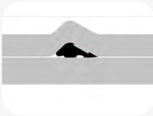
Align spigot and socket, and slide the spigot into the pipe, past the seal.
