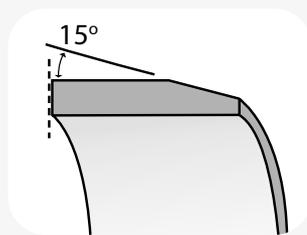
Inspect the spigot, socket and seal for damage and remove any dirt or dust prior to assembly. Chamfer the spigot end and remove all burrs.
