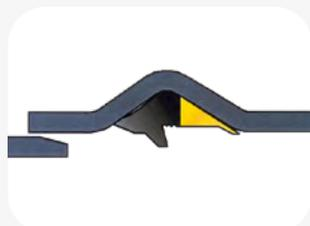
Apply lubricant to the spigot end and immediately bring it into contact with the socket.
