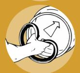
Insert the seal into the pipe and press the seal into the groove
