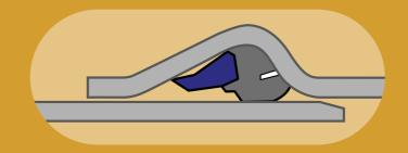
Align spigot and socket, and slide the spigot into the pipe, past the seal.
