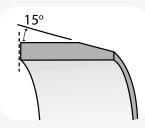
Inspect the spigot, socket and seal for damage and remove any dirt or dust prior to assembly. Chamfer the spigot end and remove all burrs.
