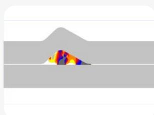
As the pipes are joined the rubber sealing element is deformed and creates pressure against both spigot and socket resulting in a watertight seal.
