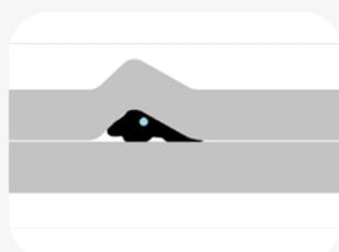
Align spigot and socket, and slide the spigot into the pipe, past the seal.
