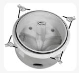
Equalize the stress in the seal by lifting and releasing at a few points. The seal must sit evenly against the spigot shoulder all around the manhole. Lubrication of the socket or spigot is not required.
