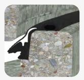
Stretch the seal onto the spigot and position against the shoulder.
