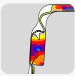
When the manhole sections are assembled, the rubber sealing element is designed to deform. This creates pressure on both spigot and socket, ensuring a watertight seal.
