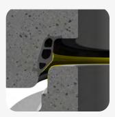
Center the socket over the spigot and lower the upper manhole element to complete the joint. Light weight elements may require an additional vertical force to fully close the joint.
