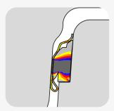
Center the spigot into the socket and assemble.
