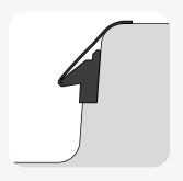
Stretch the seal onto the pipe spigot and position agains the sholder as shown. Equialise the tension by lifting and releasing the seal at several points.
