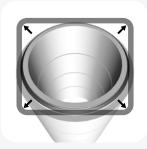
The seal must sit evenly against the spigot shoulder all around the manhole. Lubrication of the socket or spigot is not required.
