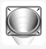
Equalize the stress in the seal by lifting and releasing at a few points. The seal must sit evenly against the spigot shoulder all around the manhole.
