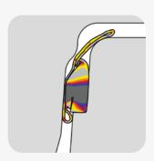
Lubrication of the socket or spigot is not required. Centre the joint and assemble. The position of the seal in the final mahole joint is shown.
