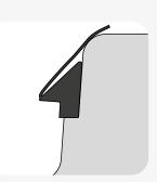
If re-joining is required ensure the sliding skin is drawn back to position as shown in picture 4.
