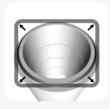
Centre the manhole sections and complete the joint. Depending on the joint design it may be possible to joint one side of the manhole, followed by the other.
