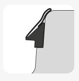
Stretch the seal onto the spigot and position against the shoulder. Equalize the stress in the seal by lifting it at a few points. It is vital that the seal seats against the shoulder around the whole circumference of the manhole.
