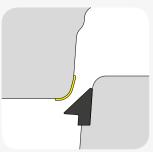
Apply lubricant to the socket. The lubricant must be evenly spread over the surface of the entire socket paying special attention to the radius at the front.
