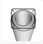
Equalize the stress in the seal by lifting and releasing at a few points. The seal must sit evenly against the spigot shoulder all around the pipe or manhole.
