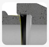
Ensure the spigot and socket are clean. Apply lubricant to the spigot. This should be spread evenly over the entire surface paying special attention to the front radius of the spigot.
