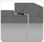
Center the spigot into the socket and push the pipes together. The socket design and wedge shaped seal provide a funnel action and help center the pipes.
