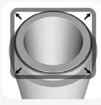
Equalize the stress in the seal by lifting and releasing at a few point. The seal must sit evenly all around the pipe.
