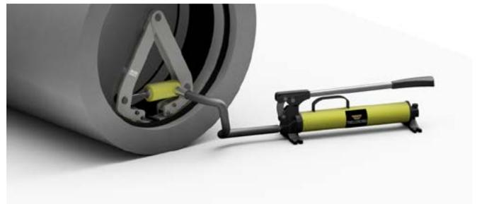
Depending on the diameter of the pipe being sealed, there will be between one and three Steel Expansion Bands and Spacer Inserts to ensure an even distribution of compressive force on the rubber seal.
