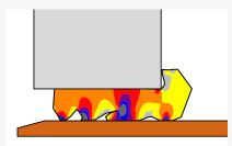
When the pipe is pushed into the manhole the rubber sealing element is designed to deform. This creates pressure on both spigot and socket, ensuring a watertight seal.
