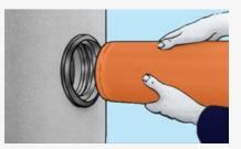
Center the spigot of the pipe and push it into the seal until the pipe end is flush with the inner wall.
