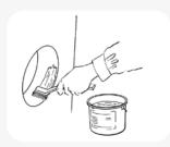
Lubricate the drilled or prefabricated hole using Trelleborg 992 Lubication.
