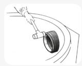
Place the seal in the hole and tap it into the correct position using a rubber or plastic mallet. Tap the end of the short plastic supporting ring that is fitted in the seal.
