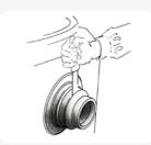
Decide which size collar is appropriate for the connecting pipe. Cut away the surplus part of the coupling using a knife. A special recess is provided for this purpose.
