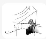
Lubricate with a thin coat of Trelleborg 992 Lubrication over the rubber part. Connect the pipe and fit the clamping band in place. Tighten the screw so that the rubber is compressed against the connecting pipe.
