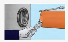
Chamfer the edge of the connecting pipe and lubricate it with Trelleborg 992 Pipe & Manhole Lube.
