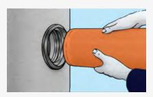
Center the end of the pipe and push it into the seal, the pipe end is flush with the inner wall.
