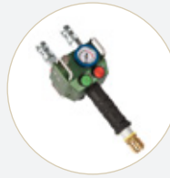
HAND-HELD DOUBLE DEADMAN CONTROLLER 10 bar (145 psi) 1.6 kg (3.6 lbs) 291257
