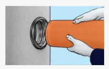
Center the spigot of the pipe and push it into the seal until the pipe end is flush with the inner wall.
