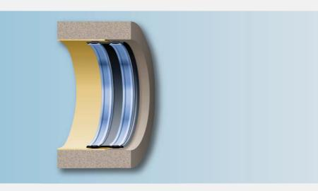
In the event that the section of host and renewed pipe adjacent to the manhole is not fully lined or cannot be completely sealed the epros®DrainLinerEndSeal is an appropriate solution. It assures the end of the liner is fully sealed and will not allow infiltration/exfiltration or root intrusion into the pipe at the sealed end.
