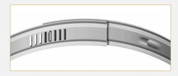
The band is then expanded using a hydraulic expansion tool. As the band expands the integral latching mechanism progresses from slot to slot, positively locking on each one until the next one is reached. There is an audible click created by the spring/rubber interaction as the band is expanded into place.
