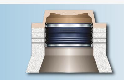
The grade adjustment area of the manhole is the first to suffer deterioration caused by freeze/thaw cycles, traffic loading, thermal expansion and contraction of the surrounding pavement and other external forces.
