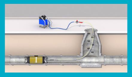
When the Trelleborg DrainPacker has reached the correct position in the pipe, it is gradually inflated using compressed air. This causes the packer to expand and press the impregnated fiberglass mat against the pipe wall. This creates a tight-fit, permanent bond against the host pipe, with the excess resin penetrating into the pipe's damaged areas (cracks and voids).
