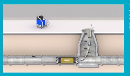
The preassembled Trelleborg DrainPacker carrying the impregnated fiberglass mat is pushed with the help of air push rods or pulled with a rope to the point of repair. The exact position of the repair point is determined beforehand through the use of a CCTV system.
