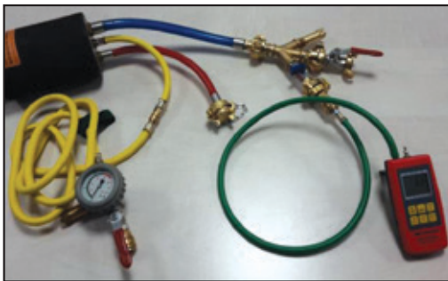
Figure 23: Air leak test with a hand-held digital pressure gauge
