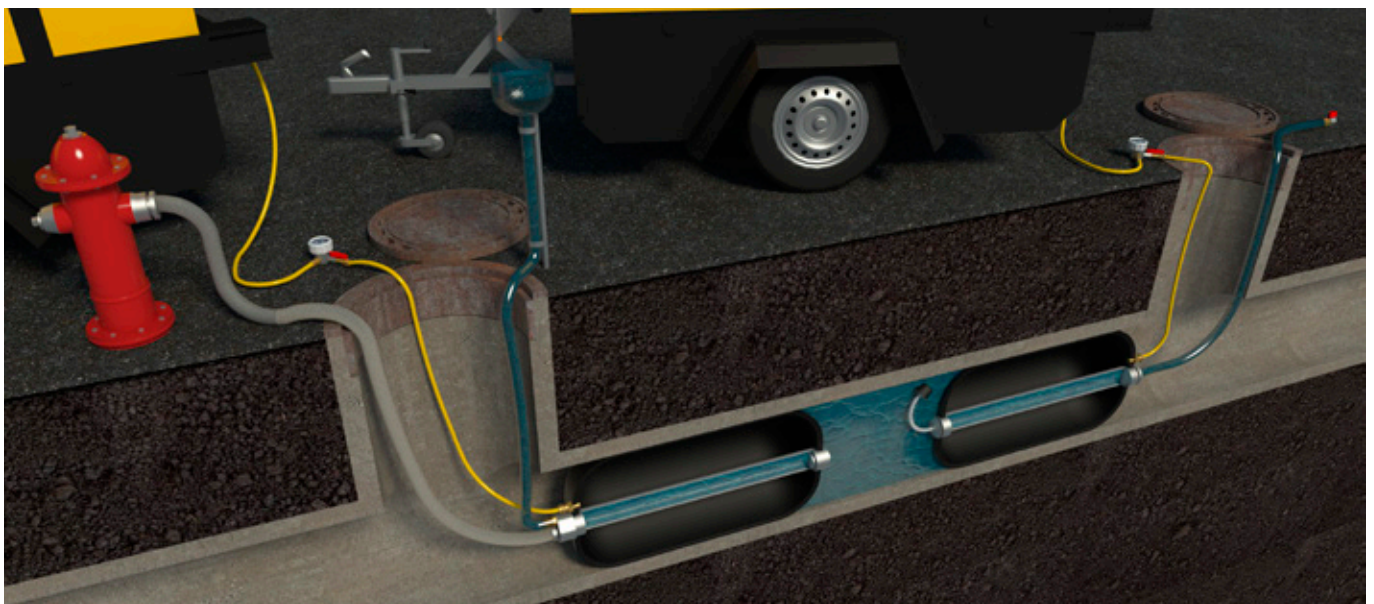
Figure 35: Water leak test of pipelines
