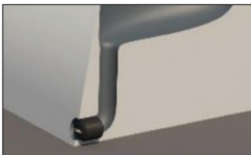
Figure 31: Inserted blocking plug
