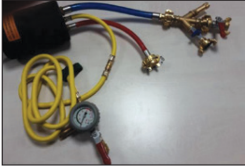
Figure 22: Connection for testing with air
