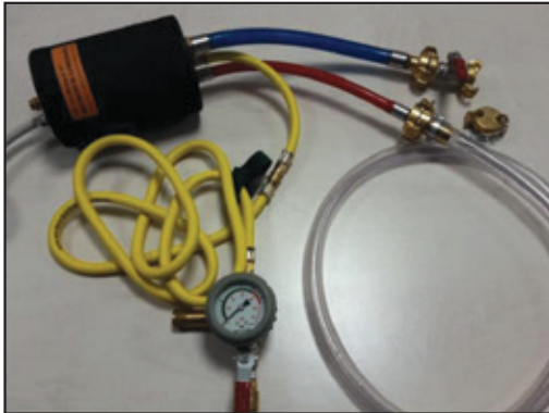
Figure 26: Connection for testing with water
