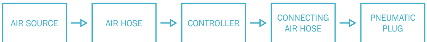
Figure 10: Pneumatic plug system
