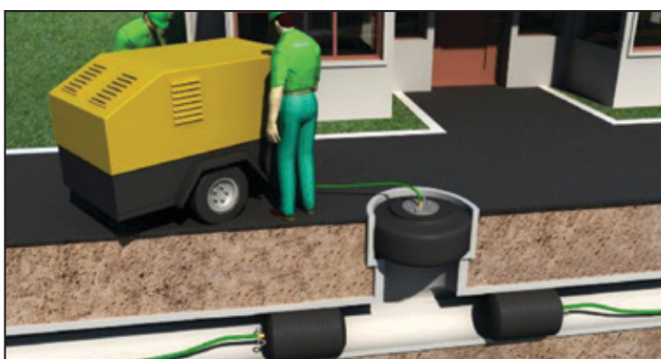
Figure 36: Gully leak test
