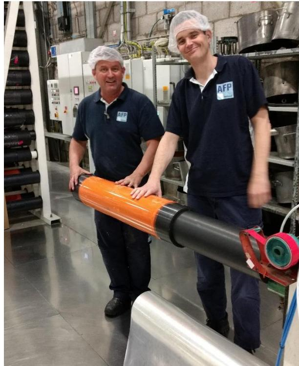
The carbon fiber bridge sleeves developed by Axcyl provide an exceptional reduction in bounce, eliminating the streaks that can so often appear in the final printed product. The pneumatically mounted bridge sleeves also have a special mounting layer that enables faster press set up.
