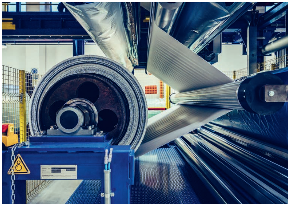
The solventless roller-head equipment during one of the manufacturing phases.
