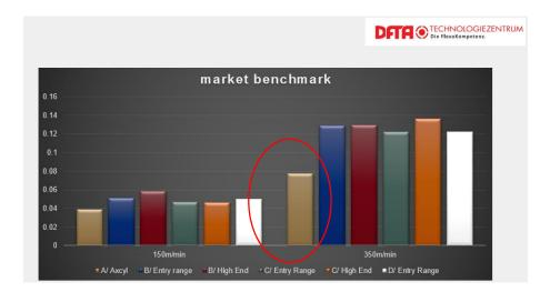
One can easily see that the Axcyl/Trelleborg sleeve Optical Density variability **is about half the variability** of other sleeve technologies, demonstrating that indeed, the Trelleborg structure dampens vibration coming from printing plate.
