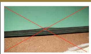
These MBB has been damaged by a wrong box opening
