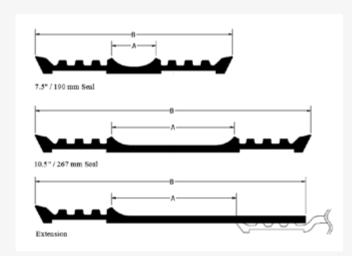
A = The portion of the seal that covers the leaking area.
